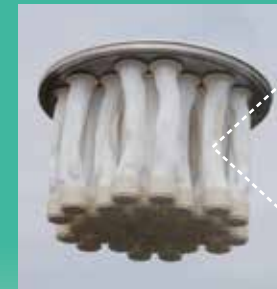
FG31 multi-module vessel inner membrane module
