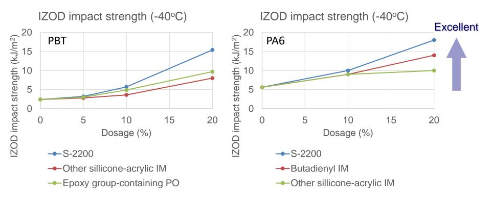
Test piece: 1/8 inch thickness, mold-notched (set value)
