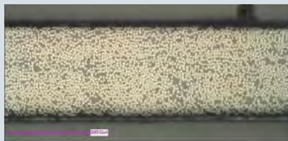
Kyron™ULTRA cross-sectional photo (enlarged from 100.0μm) This image demonstrates that the internal void is kept to a minimum.
