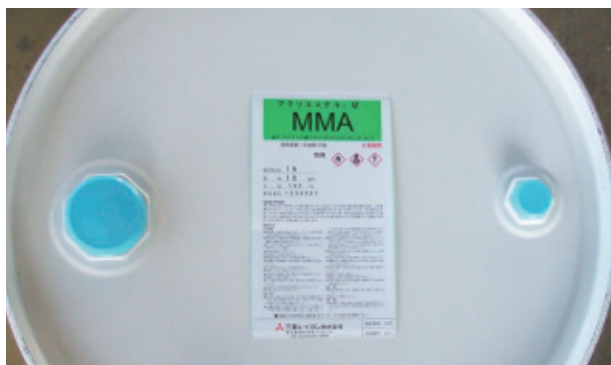
A GHS compliance form is affixed to the top of a drum containing MMA monomers
