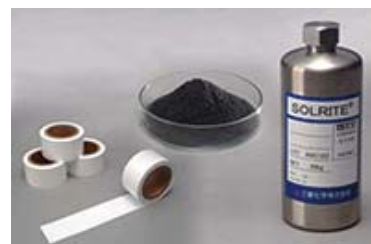
Lithium-ion rechargeable battery key materials (from right to left: electrolyte, anode material (MCC), and separator (MPI))
