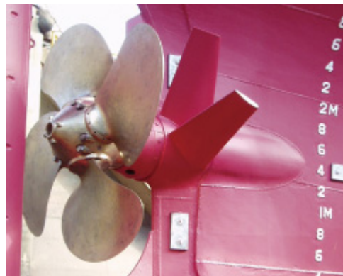
"Friend" fins added to ships to increase fuel efficiency
