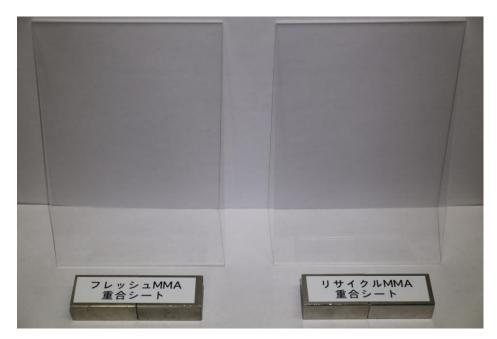
(Comparison of an ordinary acrylic plate (left) and a recycled acrylic plate (right))
