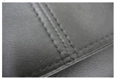
Enlarged photo of an automotive interior skin, using the new grade of TEFABLOC™ Improved moldability allows for reproduction of stitching patterns with a molding process, offering a more realistic appearance.
