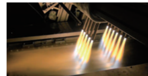
Oxy-fuel burner that contributes to reduced CO 2 emissions
