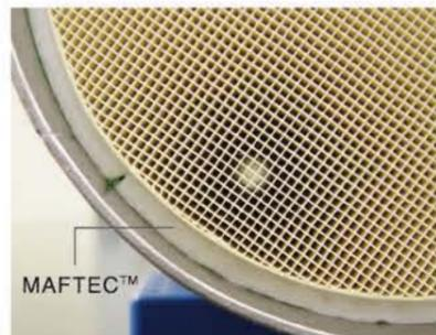
MAFTEC™ is used in automotive catalytic converters
