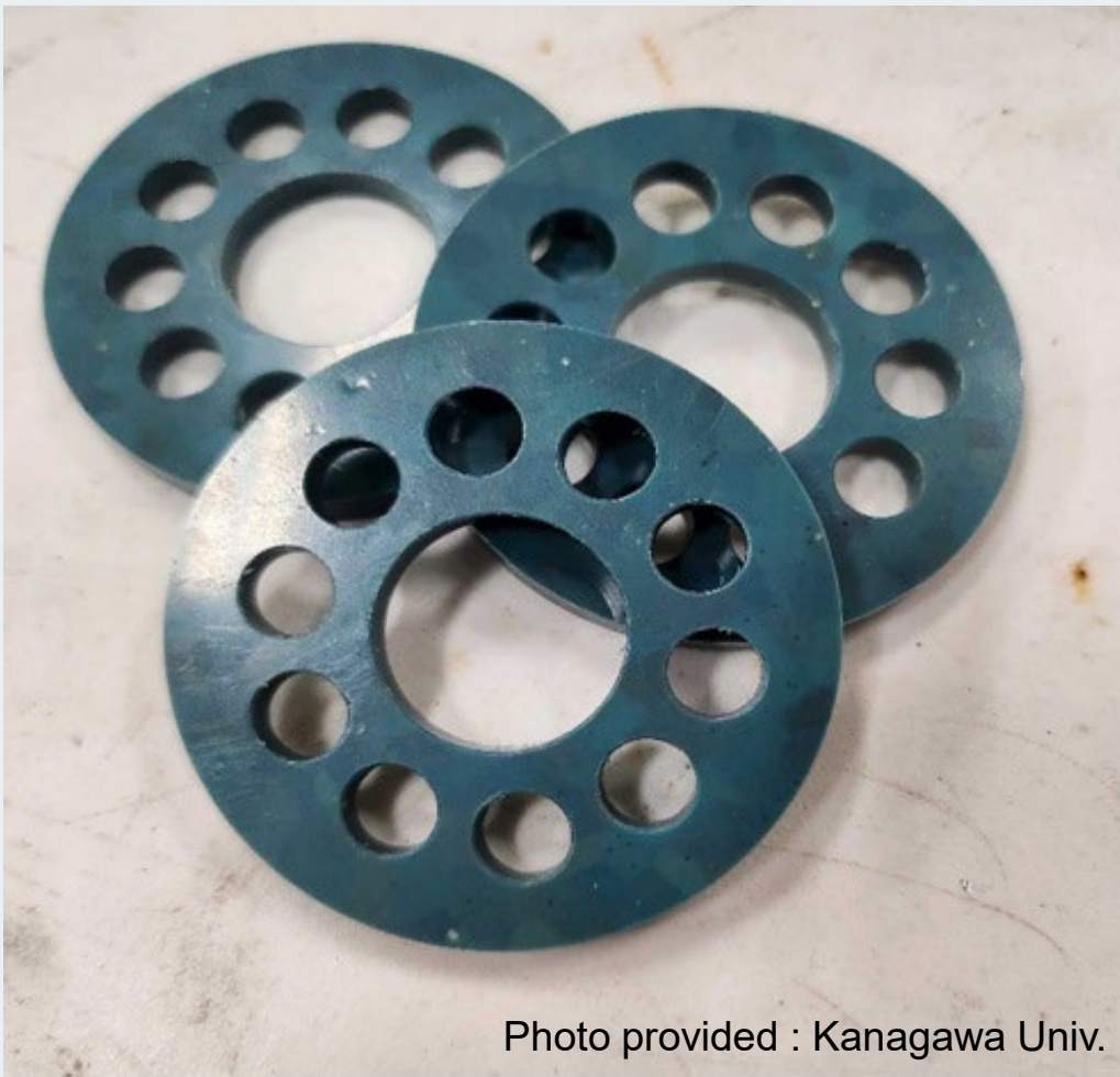
Oceanic plastic (PE) molded for fuel (Provided by: Shinshu University Nakayama Laboratory)
