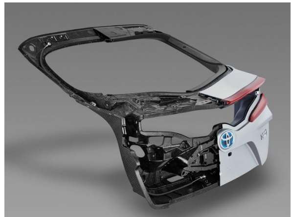
【MRC's SMC adopted by the rear door frame of the new Prius PHV】
