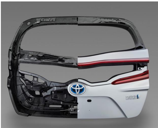
【MRC's SMC adopted by the rear door frame of the new Prius PHV】
