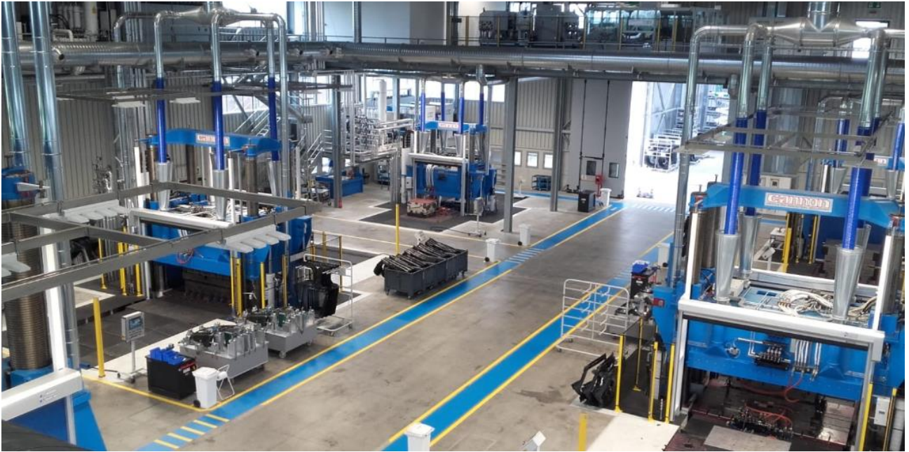
5,000-metric ton press machines at CPC
