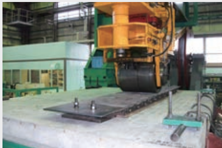
Wheel load running test
