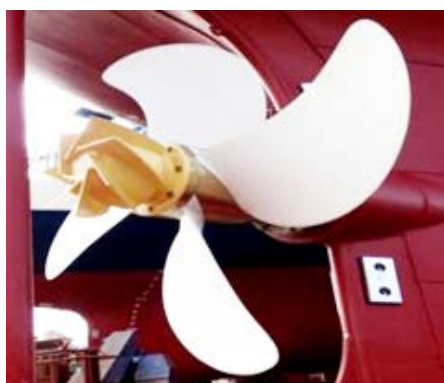
Propeller made with carbon fiber
