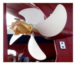
Propeller made with carbon fiber
