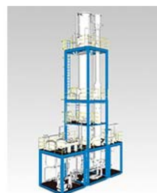
High-purity NMP recycling system used in the manufacture of lithium-ion batteries
