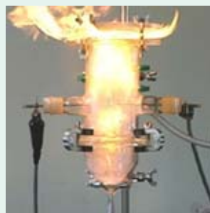
Controlled mock dust explosion experiment
