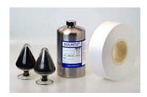
Four key materials (from left: cathode material, anode material, electrolyte, and separator)
