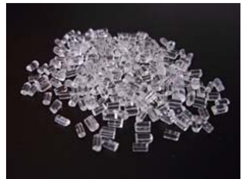
DURABIO™ transparent bio-based engineering plastic
