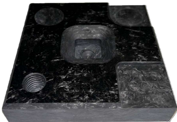
Forged Bulk Compound machined part
