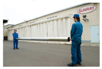
Roller for film production line (face length 9.2m, clad roller)
