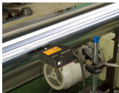
Measure Run-out by laser
