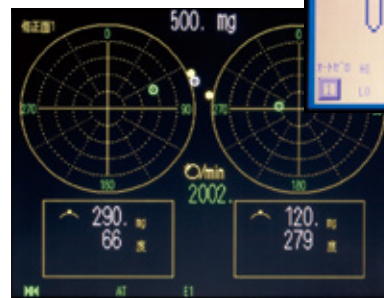
Dynamic balance at 2002rpm
