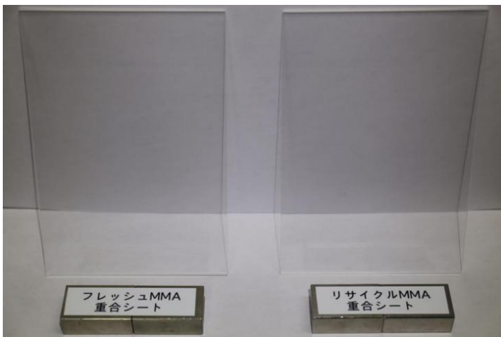
The sheet on the left is a conventional product, and the sheet on the right is a recycled product. Both have the same level of transparency.
