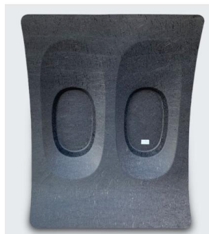
Joint development with Boeing Company of aircraft interior materials using recycled carbon fiber is in progress.
