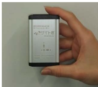
Motion Recorder with 3-Dimensional Acceleration sensor
