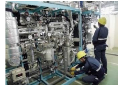
Membrane reactor of methanol synthesis (Pilot test)
