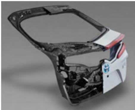
MCC's CF-SMC adopted by the rear door frame of the Prius PHV (Photos by Toyota Motor Corp.)
