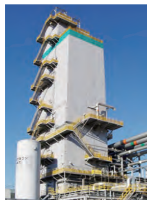
Energy-efficient, super-large air separation unit
